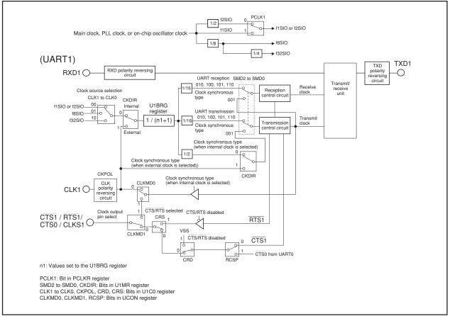
Figure 14.2 UART1 Block Diagram
